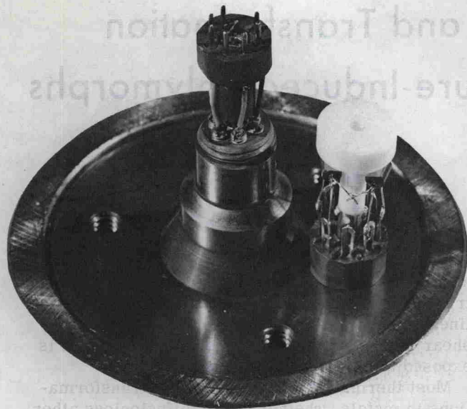
Fig. 1—Specimen holder and bottom closure for hydrostatic pressure system.
